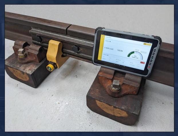
Monitoring temporary rail clamps remotely improves safety and reduces inspection!
