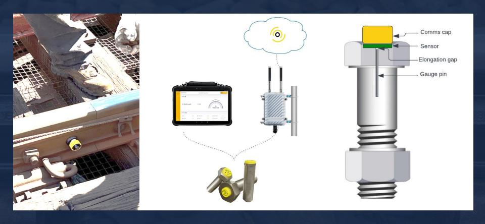
A gauge pin is fixed within the fastener using a specialised permanent bonding technique; as the bolt is stretched it creates a gap between the pin and the sensor, which the sensor measures and converts to clamp force. The bolt sends data to a gateway, within 1km, which in turn sends the data up to the Cloud, where it can be accessed through a dedicated portal on any wifi-enabled device.
